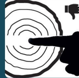
Split, where the opening is continuous and is also between 8 mm and 25 mm.
