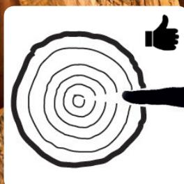
A crack that has an opening that becomes smaller towards the centre of the wood is not critical, since there is no finger entrapment hazard.
