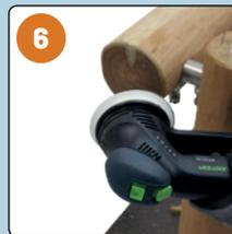
Sand the wooden wedges' exposed surface
